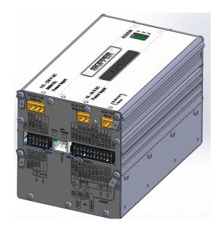
The JB70D1 housing is a versatile enclosure, containing 2 Eurocard modules. It can be mounted on DIN50 standard rails or on provided screw fastenings. Connectors are via pluggable spring connectors to the sides of the unit, with power inputs on the top row and communications on the other.
